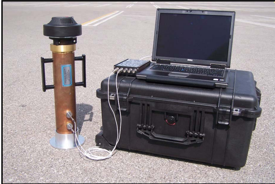
Figure 7: Stand alone system for pavement absorption measurement.
